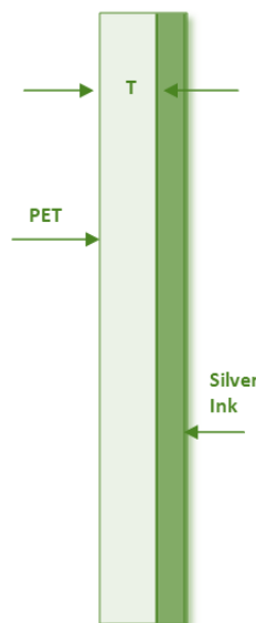
Figure 02: Side View - Proposed Concentric Hexagram Configuration of the Tamper Evident Tag
